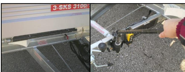
Figure 4: Lever and hand pump
